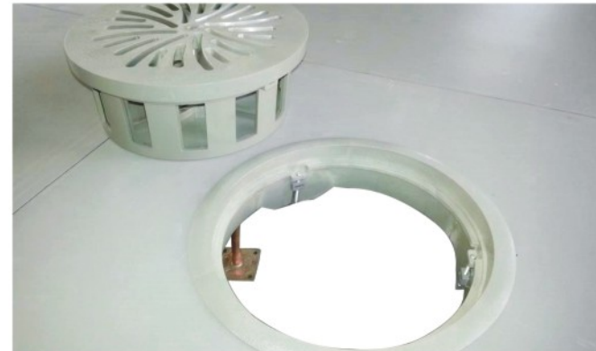
注：UFD-M-B-G散流器高度115mm，外框直径295mm，地板需要开孔圆直径265mm。 UFD-M-B-G diffuser height 115mm, frame diameter 295mm. The floor requires opening round diameter 265 mm.
