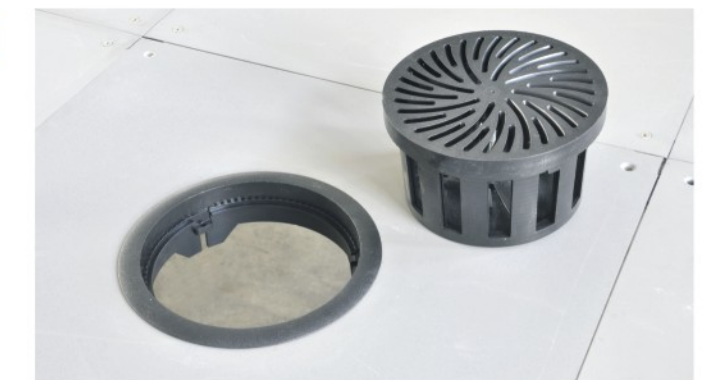
注：UFD-M-A-B散流器高度120mm，外框直径235mm，地板需要开孔圆直径205mm UFD-M-A-B diffuser height 120mm, frame diameter 235mm. The floor requires opening round diameter 205 mm.
