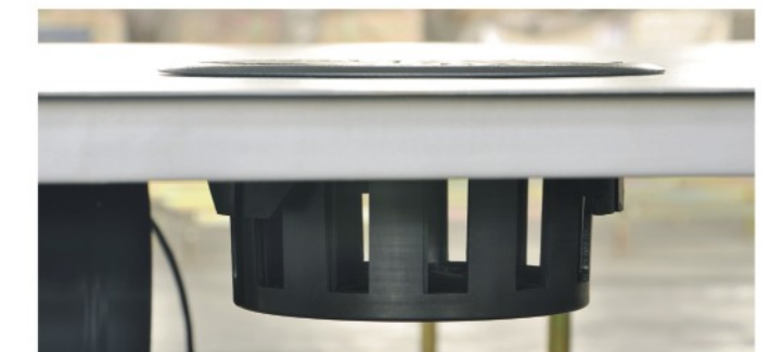
注：UFD-M-A-B散流器高度120mm，外框直径235mm，地板需要开孔圆直径205mm UFD-M-A-B diffuser height 120mm, frame diameter 235mm. The floor requires opening round diameter 205 mm.
