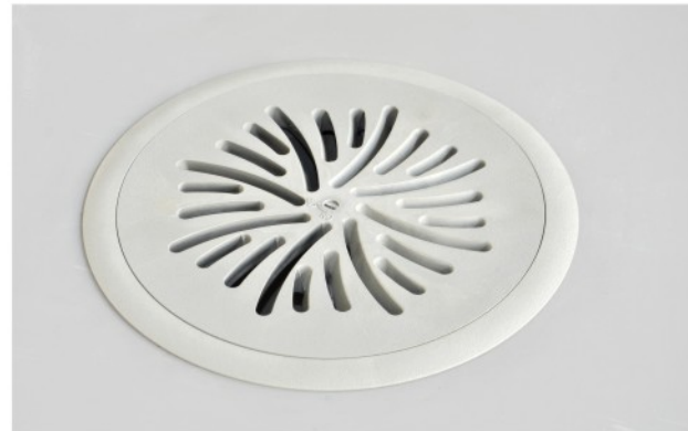
注：UFD-M-B-G散流器高度115mm，外框直径295mm，地板需要开孔圆直径265mm。 UFD-M-B-G diffuser height 115mm, frame diameter 295mm. The floor requires opening round diameter 265 mm.
